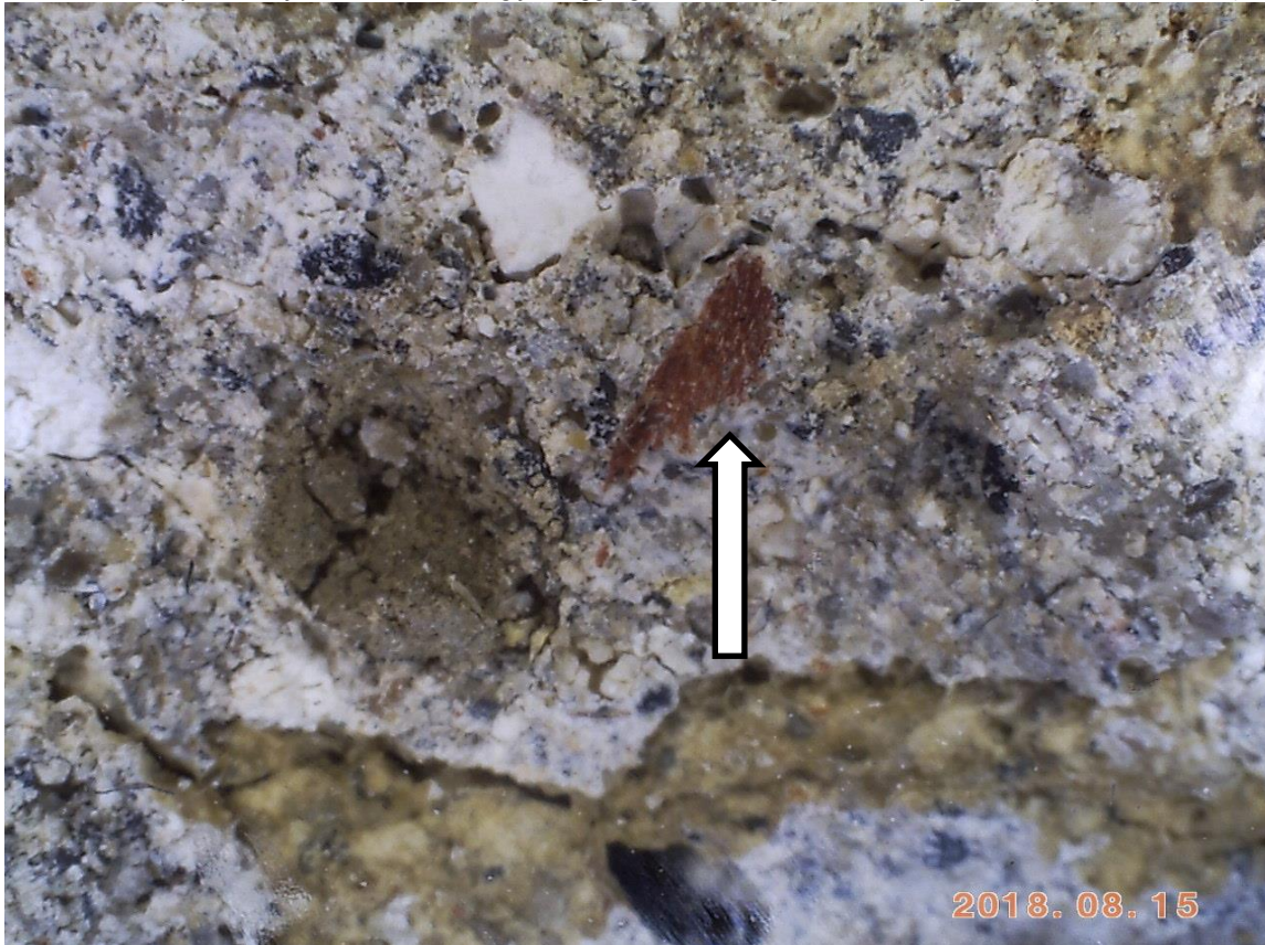
Above: Microscope detail showing clay (brown & yellow-brown) and a ceramic fragment (pozzolan, arrowed).
